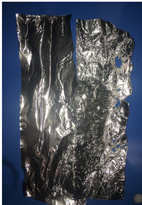
Figure 1 Powersonics™ Radial Transducer Aluminum Foil Test
